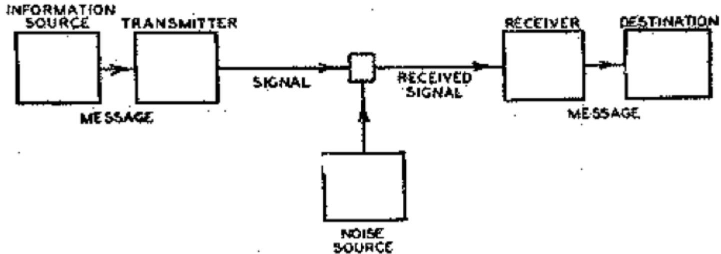
Fig. 1—Schematic diagram of a general communication system.
